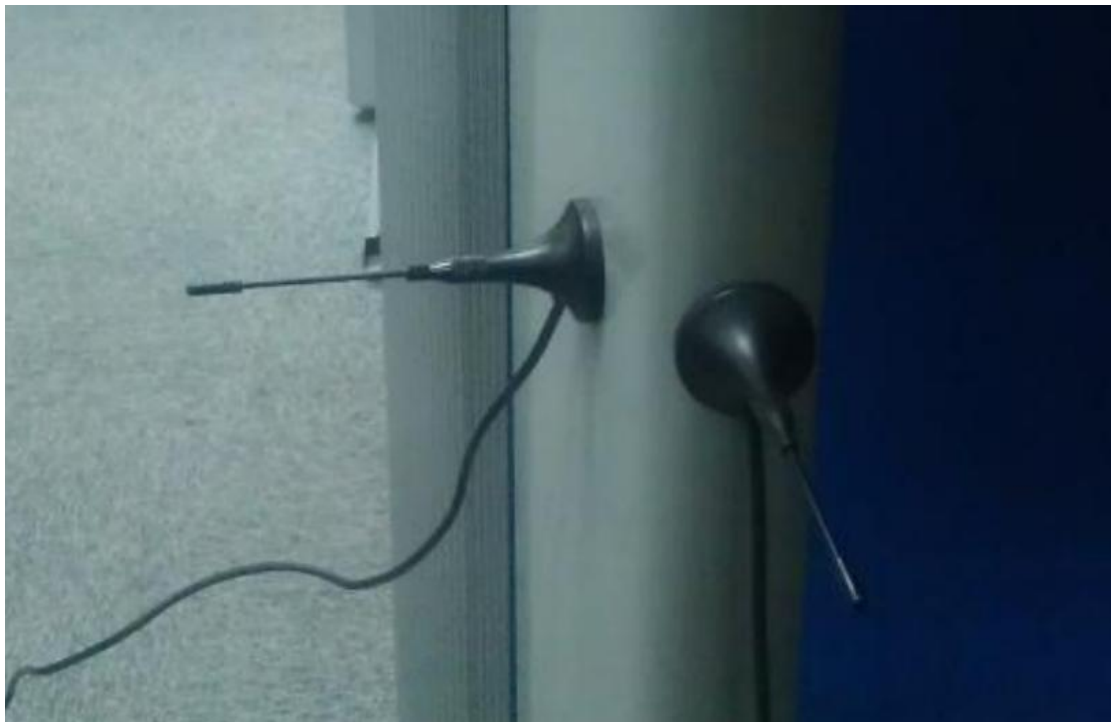
Figure 6.3 Isolation by antenna orthogonal polarization
